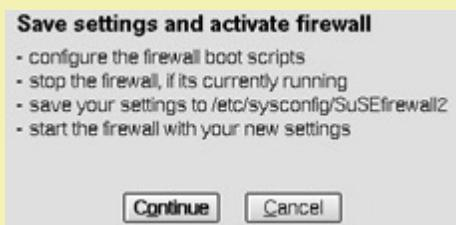
Figure 3-10: SUSE Linux Save settings and activate firewall
