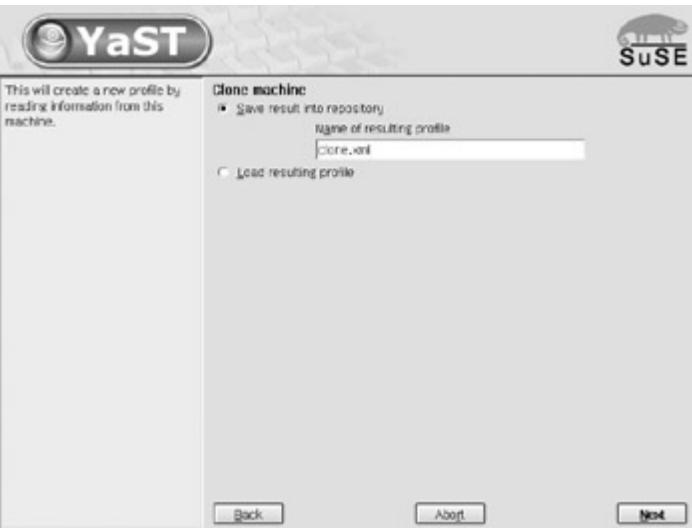
Figure 5-4: SUSE AutoYaST showing entry of the filename clone.xml
