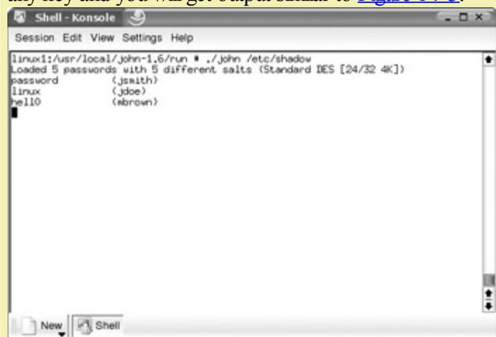
Figure 14-3: John the Ripper output
