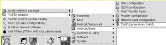
Figure 2-3: YaST2 menu hierarchy for invoking inetd services GUI
