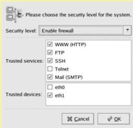
Figure 3-12: The Red Hat firewall configuration tool
