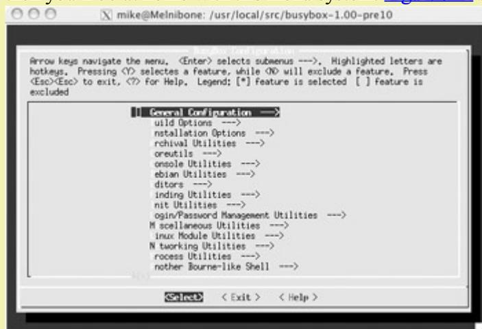
Figure 9-1: The `make menuconfig` step for BusyBox
