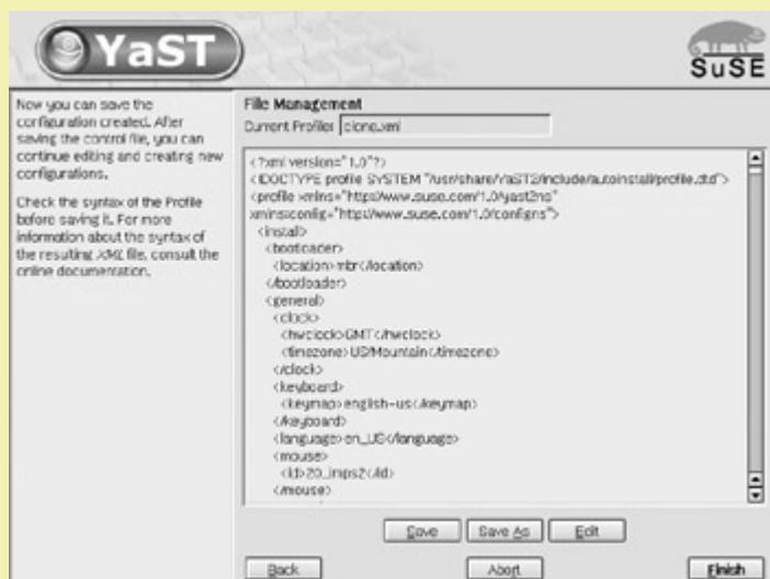
Figure 5-5: SUSE AutoYaST utility ready to save the clone.xml profile file
